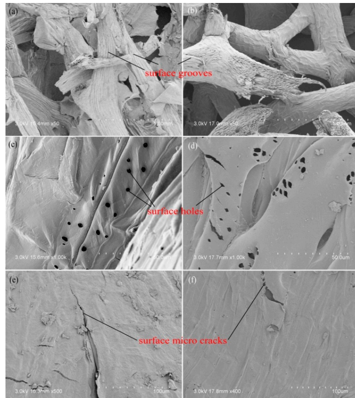
Figure 17. The surface topography of fiber bundles taken from two-density luffa sponge (a) (c) (e) are from luffa sponge of low density, (b) (d) (f) are from luffa sponge of high density.
