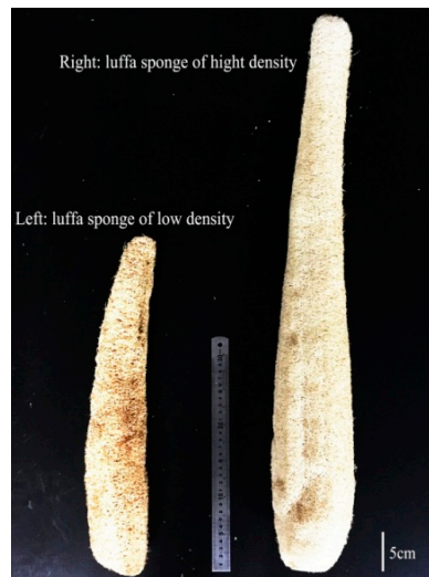
Figure 2. The luffa sponge of high density and low density (left: low density luffa sponge, right: high density luffa sponge)
