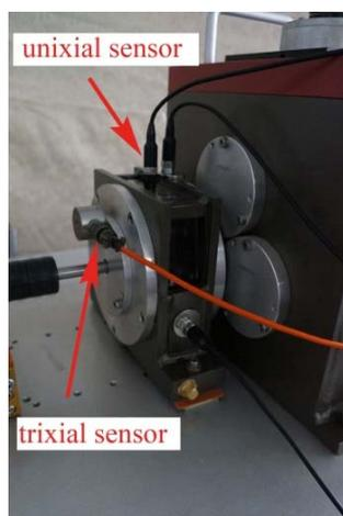
**Fig. 3.** Layout mode of acceleration sensor
