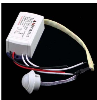
98 Figure 2. PIR-based motion sensor switch, the type used in this project [1]
