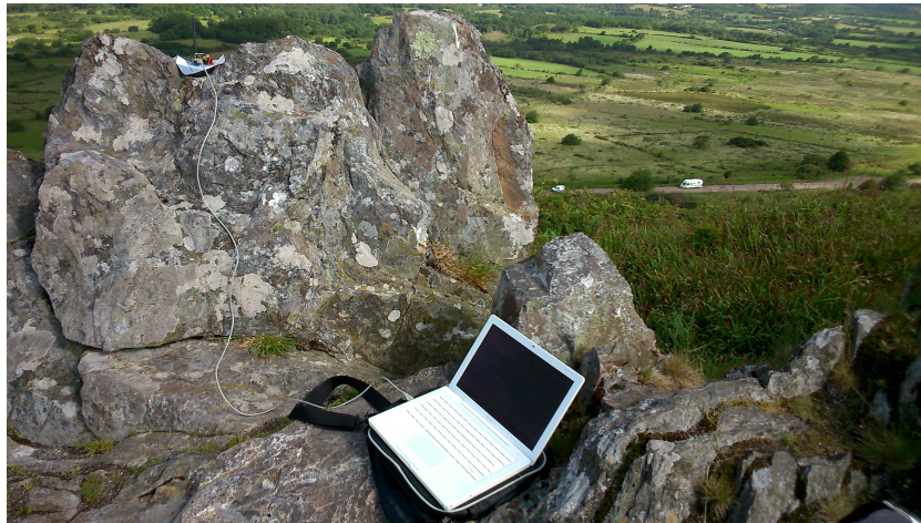
Figure A5. A base station is equipped a LoRa board (emitter) and MacBook. This base station was deployed on the top of Roc'h Trevezel mountain, France. For receiver, another LoRa board is mounted on a car moving around.
