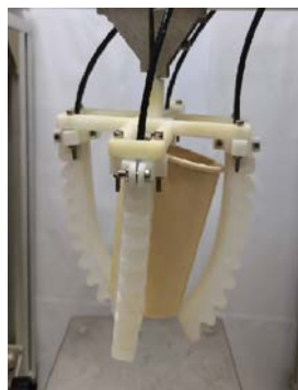
Figure 19. Test on the maximum grasped weight of the soft gripper
