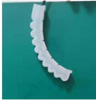
Figure 16. Air tightness check of soft actuator.
