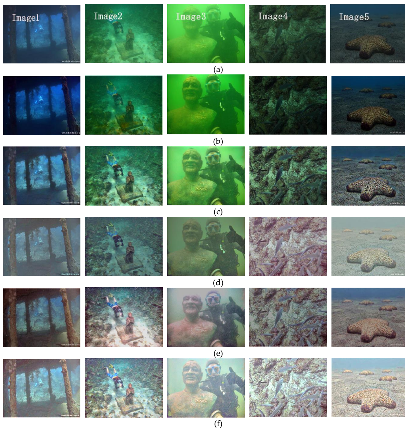
Figure 3. Comparison of experimental results with different algorithms: (a) Original images; (b) Algorithm in literature [35]; (c) CLAHE algorithm; (d) MSRCR algorithm; (e) Algorithm in literature [36]; (f) The proposed algorithm in this paper.
