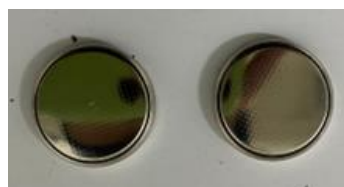
Figure 8. Supercapacitor coin cell device with \text{Na}_2\text{SO}_4 electrolyte solution.
