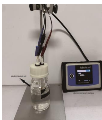
Figure 4. Scheme of measurement with a three-electrode system. (a) measurement models, (b) real time measurements, and (c) electrochemical cell components.
