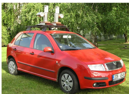
Figure 1. A car with universal doubled jet spore sampler.
