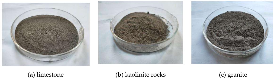
Figure 2. Three types of mineral powder samples: (a) Clayey, (b) Limestone, and (c) Granite.
