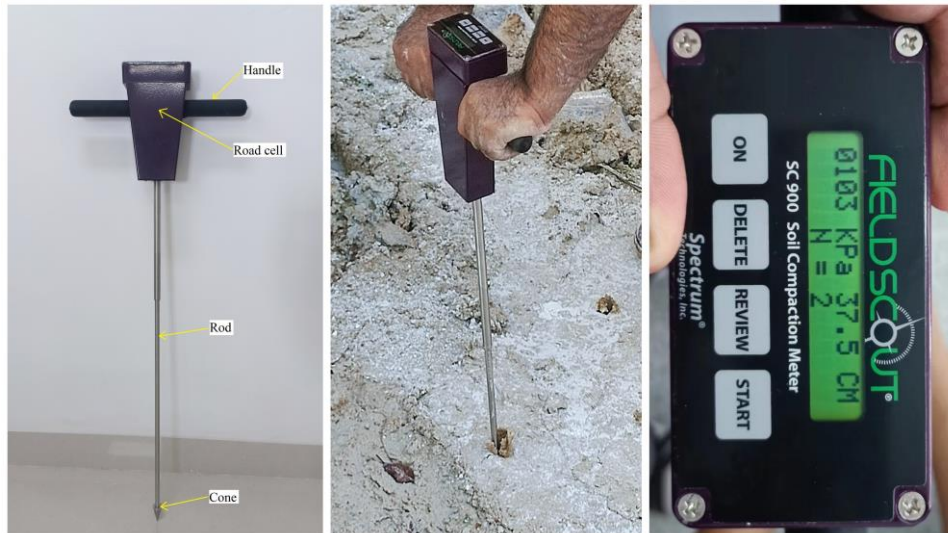
Figure 2. Cone penetrometer and sampling by cone penetrometer.
