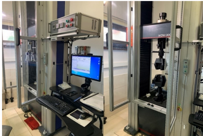
Figure 1. Testing setup for static tension testing of samples cooled after surviving a simulated fire incident.
