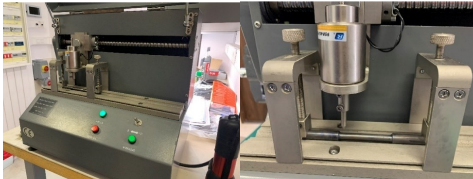
Figure 3. Marking of the initial (base) measurement length on a sample.
