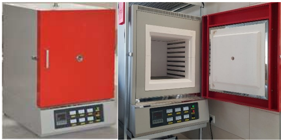
Figure 6. KJ-M1200-64L-IC muffle furnace used in the experiment to heat the tested samples in simulation of a fire incident.
