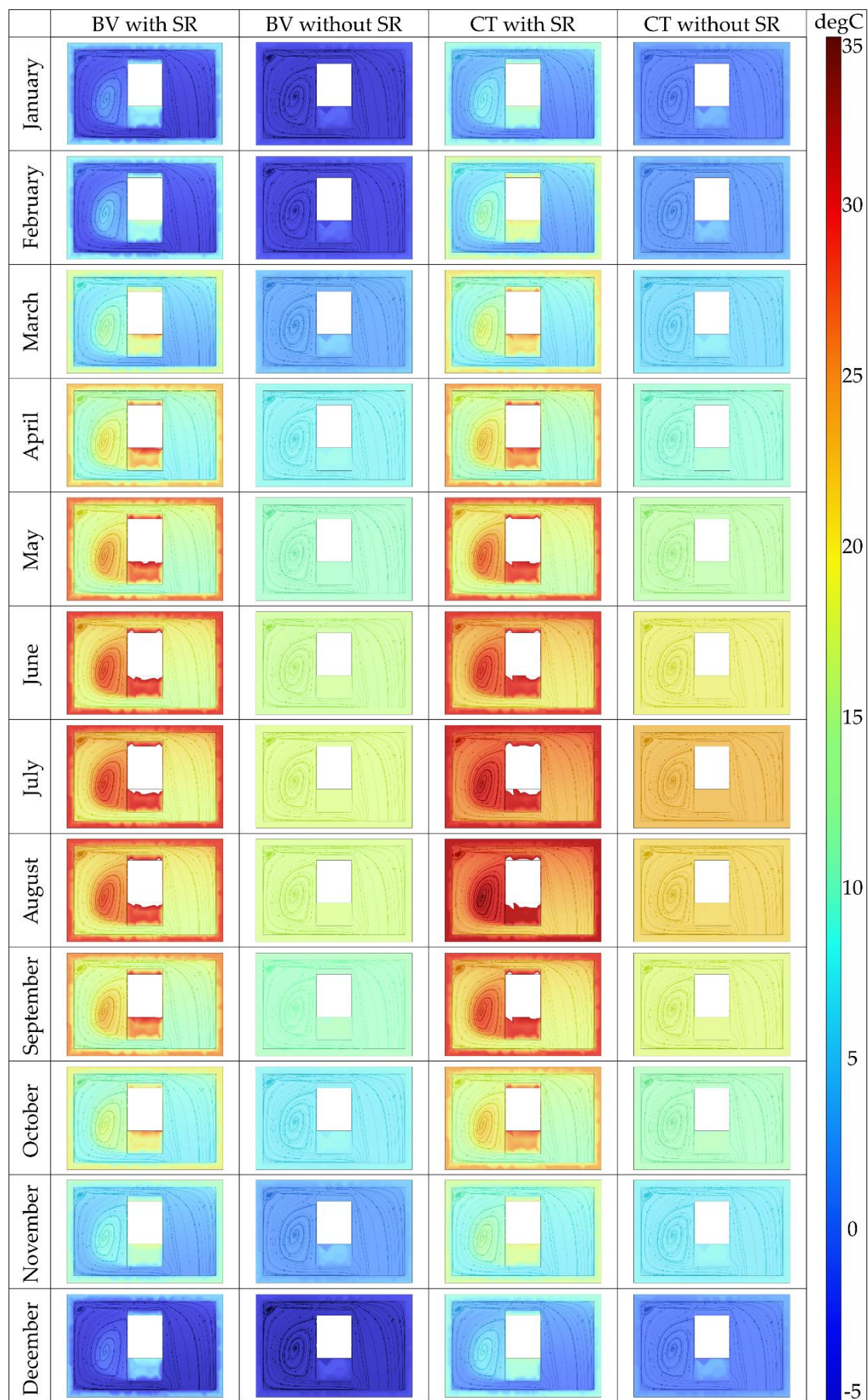
Figure 13. Cross-sections through air cavities for all 4 cases representing temperature variation.
