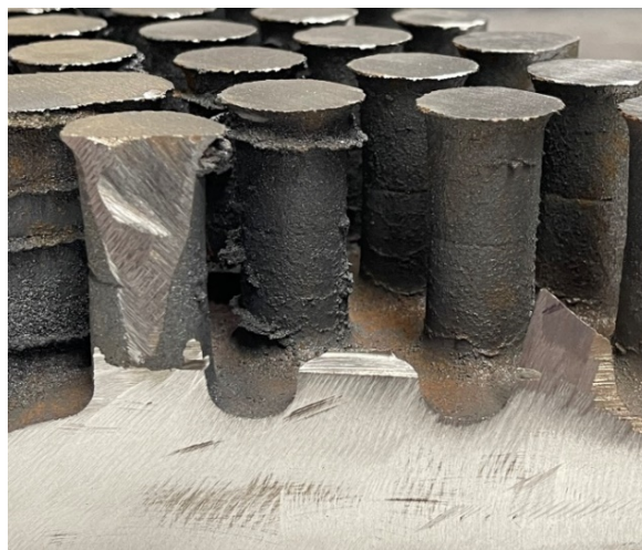
Figure 14. Cut of the casting in the critical area (without shrinkages).
