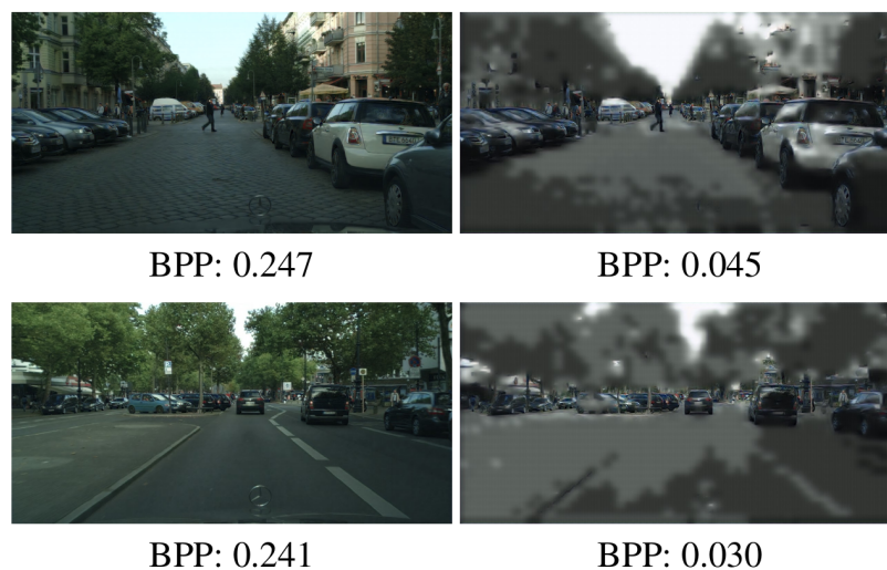
Figure 16. Reconstructed images of Le's approach for Instance Segmentation, cited from [143]. Note that at a low bitrate, the background will be severely suppressed.
