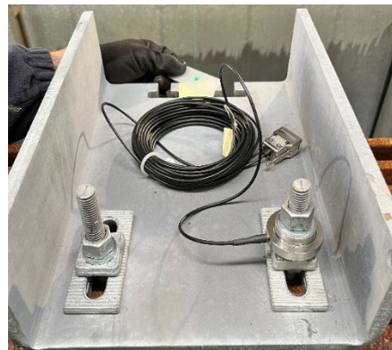
Figure 14. Façade bracket with force washer installation.
