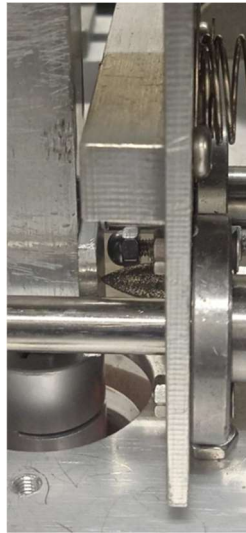
Figure 6. Scratching test of extruded aluminum using pin and round heads.
