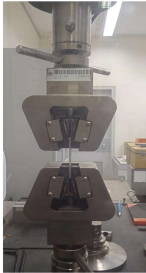
Figure 8. Tensile test of extruded aluminum sample.
