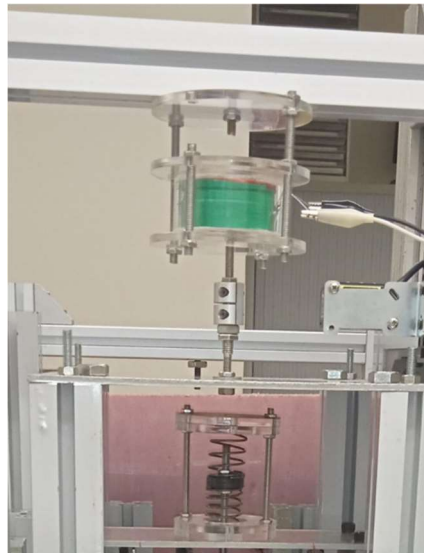
Figure 2. Electromagnetic exciter and its mounting to system mass.
