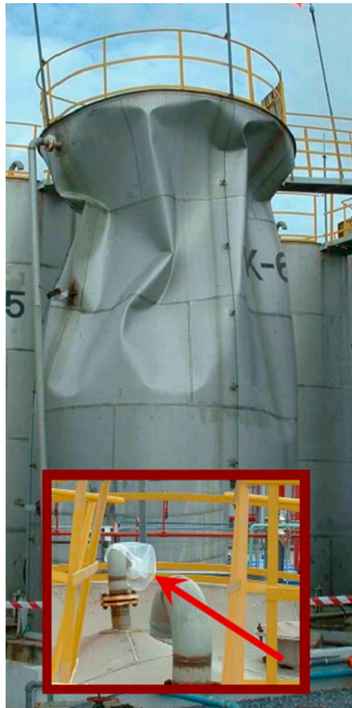
Figure 3. An example of a pressure vessel collapsing due to a plastic sheet blocking a vent [15].
