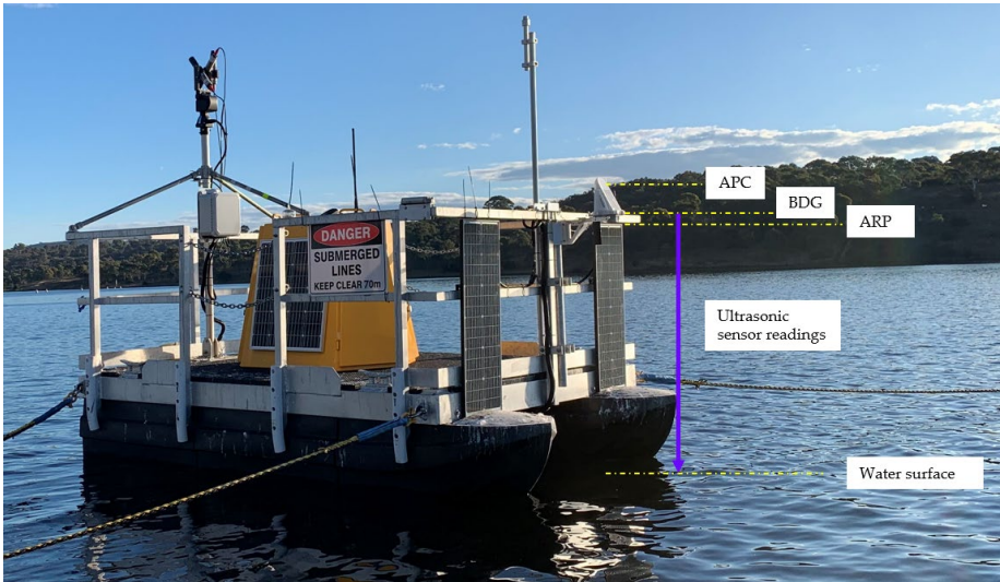
Figure 6. Experimental set-up on the CSIRO Dark-water Inland Observatory Network’s pontoon at Googong reservoir (photo credit: D. Culvenor and G. Kerrisk).
