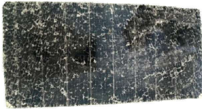
Figure 1. Test sample from an obsolete single-sided PV panel.
