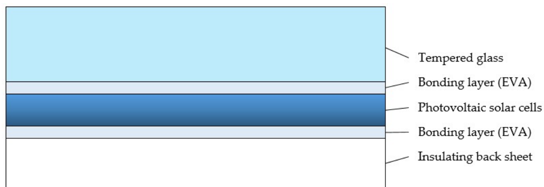
Figure 2. Scheme of the cross-sectional structure of the panel used for the tests.
