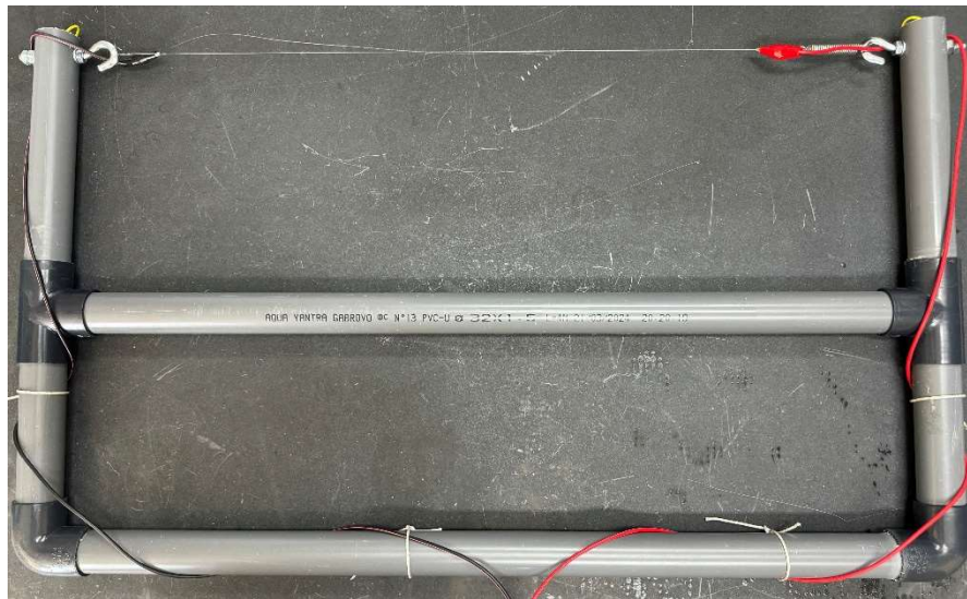
Figure 3. Manual proof-of-concept test device with a metal wire.
