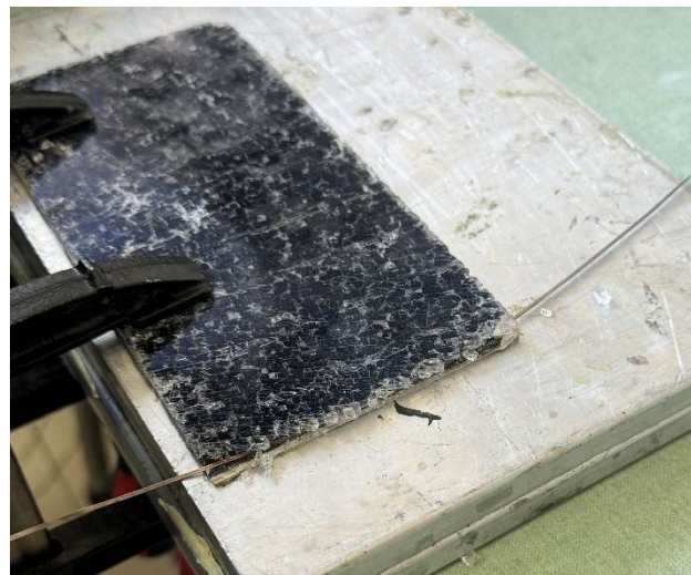
Figure 6. The wire threaded into the EVA layer between the glass and the photovoltaic solar cells.
