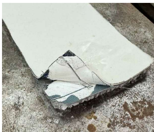
Figure 8. Partially separated insulating back sheet.
