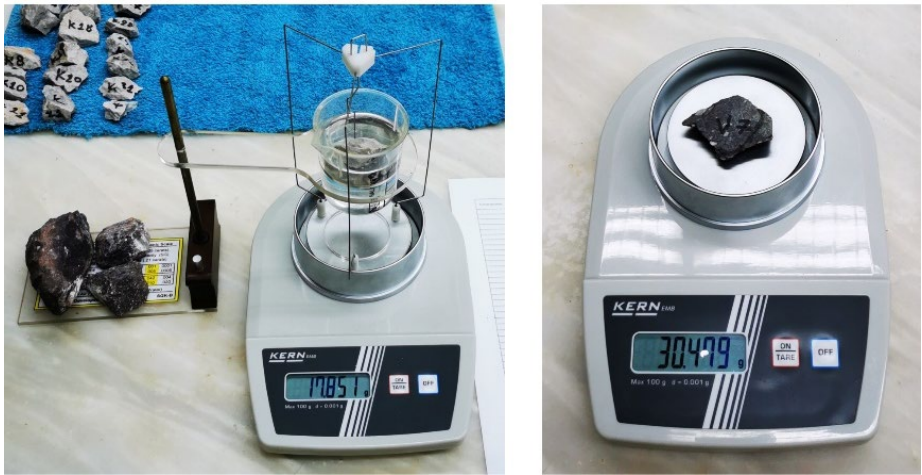
Figure 8. Laboratory measurements for density determination of geological formations.
