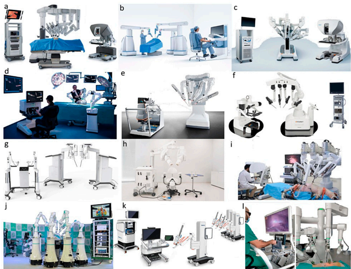
Figure 1. Most advanced RAMIS systems, featuring only commercially available, and ready-to-launch platforms, already cleared for at least a limited set of surgical indications (presented in the order of time of appearance). (a) da Vinci Xi. (b) Senhance Surgical Robotic System. (c) Revo-i. (d) Versius. (e) Avatera. (f) Hinotori. (g) Dexter. (h) Symani Surgical System. (i) Toumai Endoscopic Robot. (j) Mantra. (k) Hugo RAS System. (l) Bitrack. Table 1 at the end provides details regarding these robots’ basic engineering and clinical capabilities. (Image credit: the respective manufacturers.).
