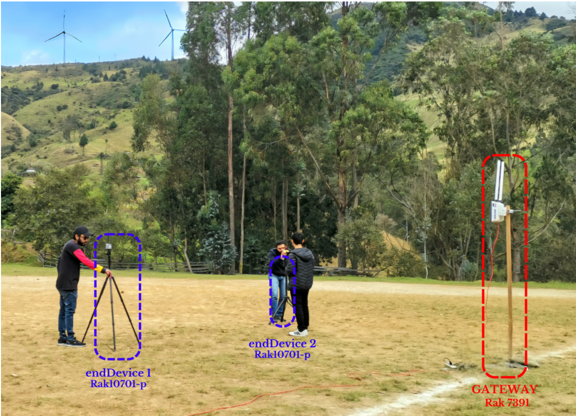
Figure 10. Experimental setup showing the gateway and end device in a suburban open area.
