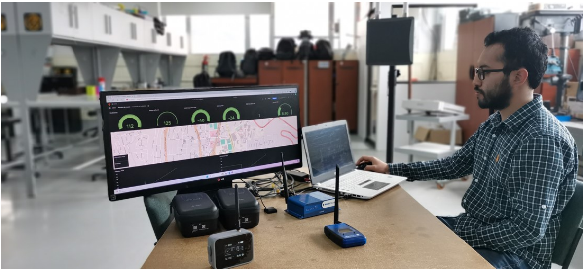
Figure 12. LoRaWAN link statistics for analysis and its presentation in the dash board in the Lab.
