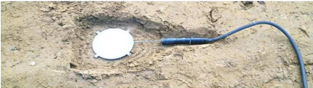
Figure 7. View of the recess prepared for the installation of the pressure transducer.
