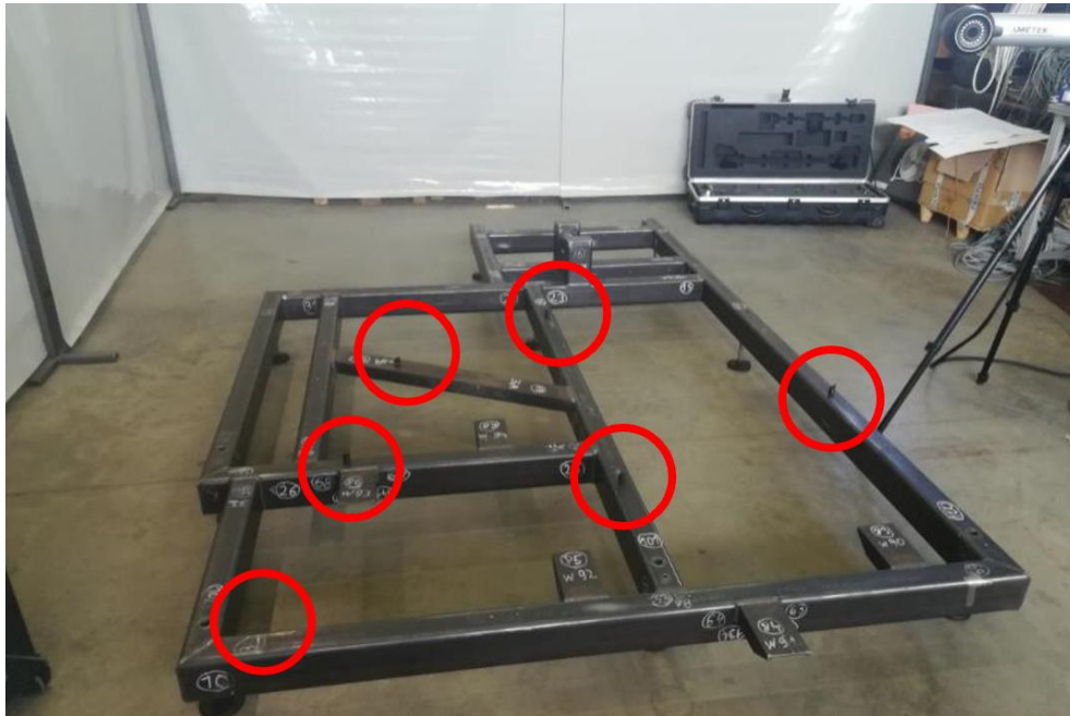
Figure 4. Example of the location of reference points on the tested frame No. 1.
