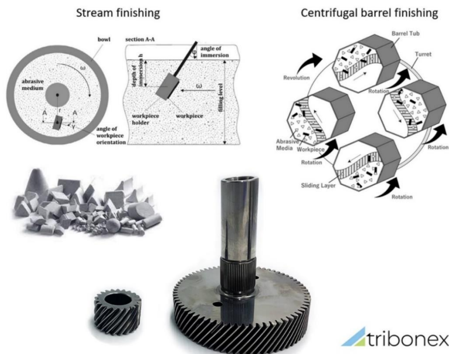
Figure 2. Examples of mass-finishing platforms used for Triboconditioning® CG treatment.
