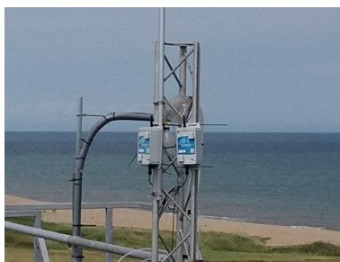
Figure 1. View of the co-located equipment at WAO: cost-effective devices 5158 and 5178 are the two blue and grey boxes
