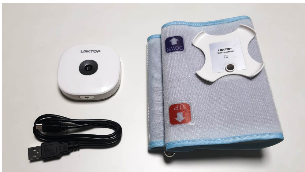
Figure 4. 6-in-1 Remote Health Monitor. The figure presents the 6-in-1 Remote Health Monitor with its cuff for blood pressure measurements and a charging cable.
