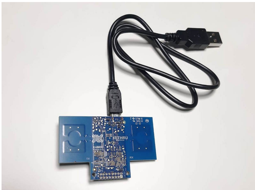
Figure 5. XeThru X4M200 respiration sensor. The figure illustrates the XeThru X4M200 respiration sensor, along with a micro USB cable for powering the device.
