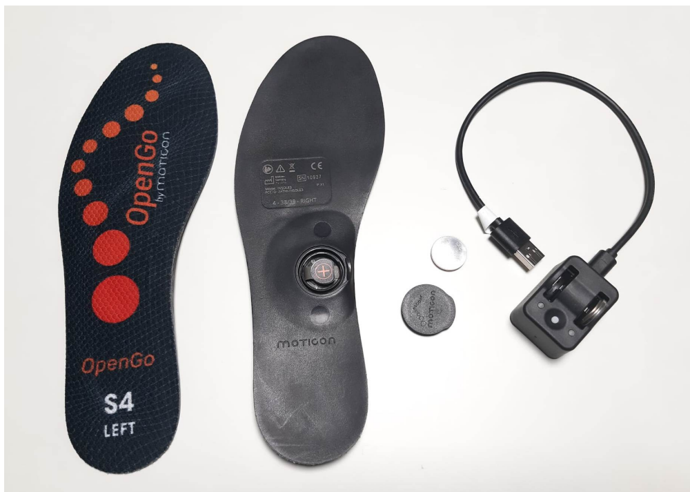
Figure 2. OpenGo Sensor Insoles. The figure presents a pair of OpenGo Sensor Insoles, showing both top and bottom views, with the battery lid and coin cell battery removed, along with the charging dock featuring an inserted battery for recharging.
