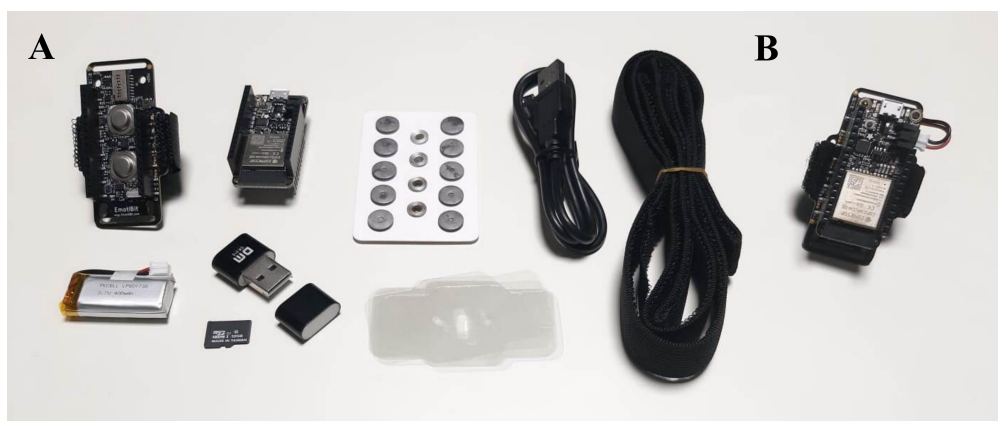
Figure 1. EmotiBit components and assembly. (A) The complete EmotiBit bundle, including the EmotiBit MD board, Adafruit Huzzah32 Feather, 400mAh lithium ion battery, high-speed microSD card, microSD card reader, electrode kit, Emoti-genic covers, micro USB cable, and Emoti-stretch straps of varying lengths. (B) The fully assembled EmotiBit.
