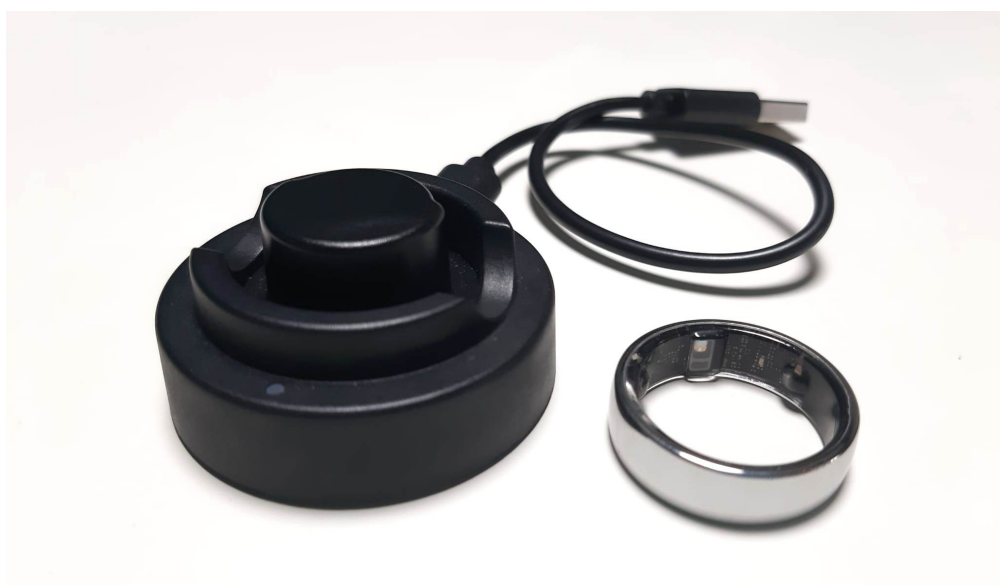
Figure 3. NexRing. The figure illustrates NexRing with its wireless charging dock.
