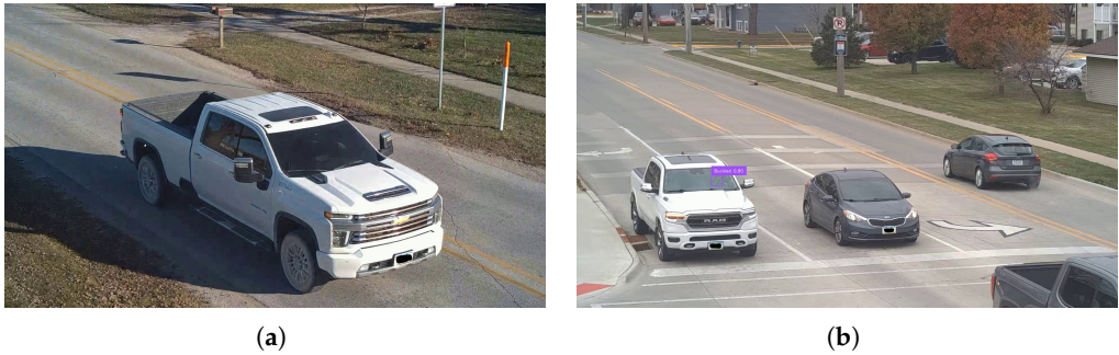
Figure 6. Missed Detections—(a) Extreme windshield tint prevented detection; however, this case was excluded from analysis, as discussed in Section 3.4. (b) seatbelt detected with high confidence on the left vehicle, but missed on the right due to heavy tint and low lighting.
