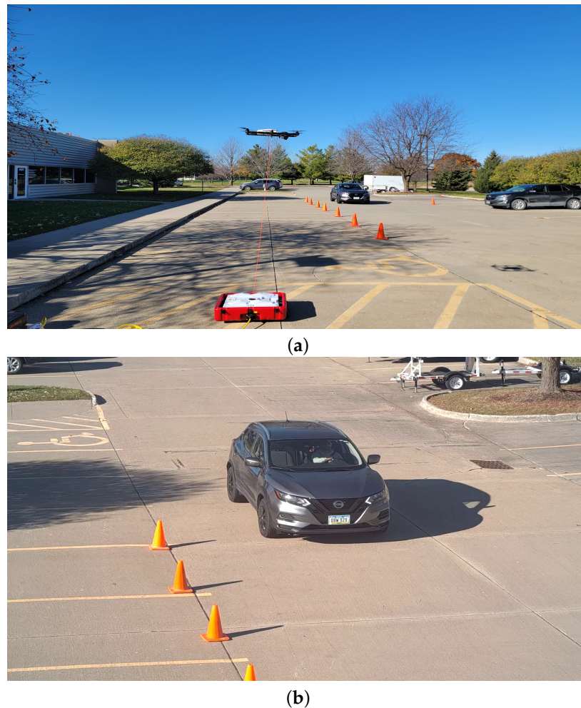
Figure 1. Experimental setup during data collection. (a) The drone mounted for aerial recording. (b) Sample output from the drone's camera after mounting and zoom adjustment.
