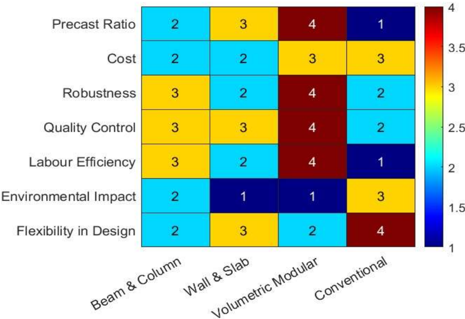
Figure 5. Heatmap comparing (Beam & Column, Wall & Slab and Volumetric Modular) Precast Systems and Conventional Construction systems across key parameters (1 = Low, 4 = Very High).
