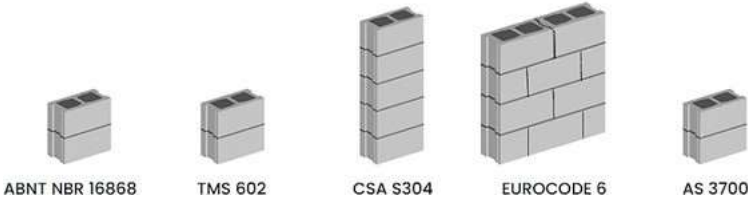
Figure 1. Masonry specimens according to different standards. Adapted by the authors from [27].
