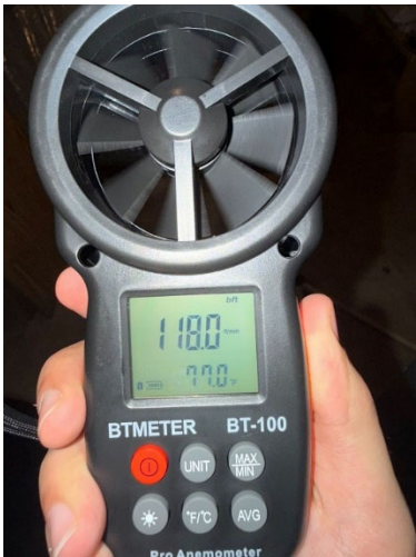
Figure 8. Maximum Airflow Test Nearest to Duct Outlet (Test 4). Airflow: 0.60 m/s (118.0 fpm). Temperature: 298.15 K (25.0°C) (displayed as 77.0°F in the figure)
