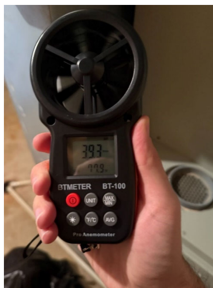
Figure 6. Intermediate Airflow Test Closer to Ductwork (Test 2). Airflow: 0.20 m/s (39.3 fpm). Temperature: 298.65 K (25.5°C) (displayed as 77.9°F in the figure)
