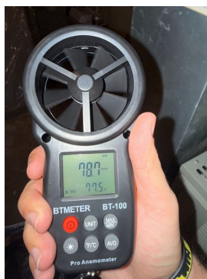
Figure 7. Increased Airflow Test in Proximity to Ductwork (Test 3). Airflow: 0.40 m/s (78.7 fpm). Temperature: 298.45 K (25.3°C) (displayed as 77.5°F in the figure)
