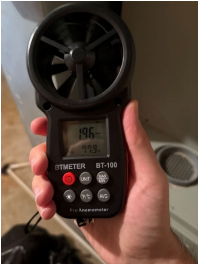
Figure 5. Initial Airflow Test at Distance from Ductwork (Test 1). Airflow: 0.10 m/s (19.6 feet per minute (fpm)). Temperature: 298.65 K (25.5°C) (displayed as 77.9°F in the figure)
