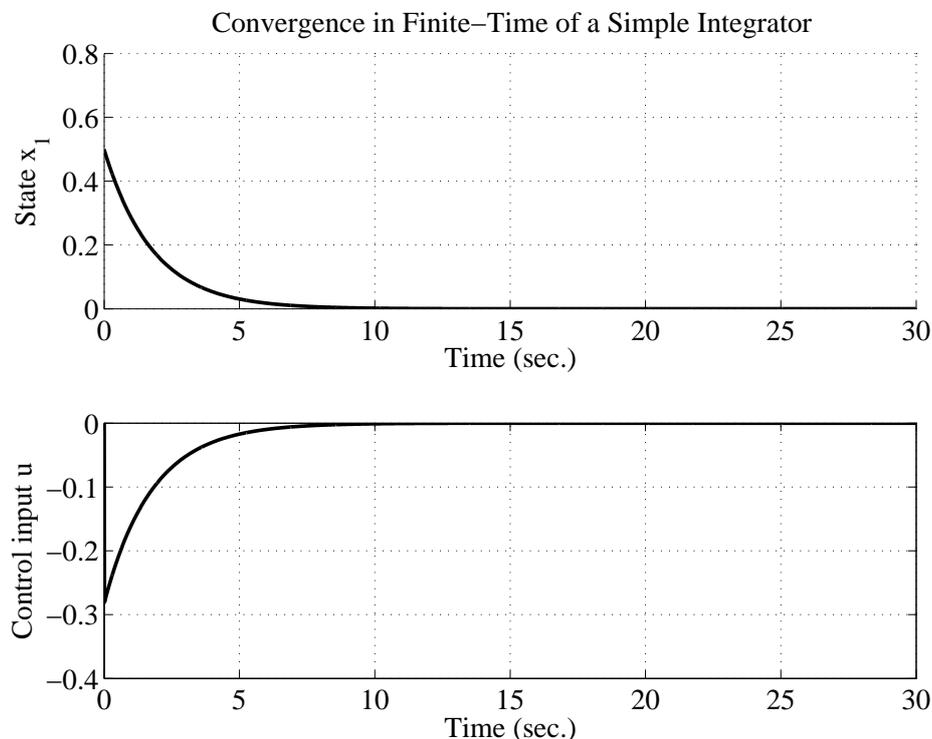
**Figure 1.** Initial condition response of a finite-time stabilized simple integrator
