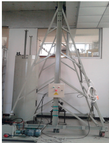
Figure 2. The air shock wave generator.
