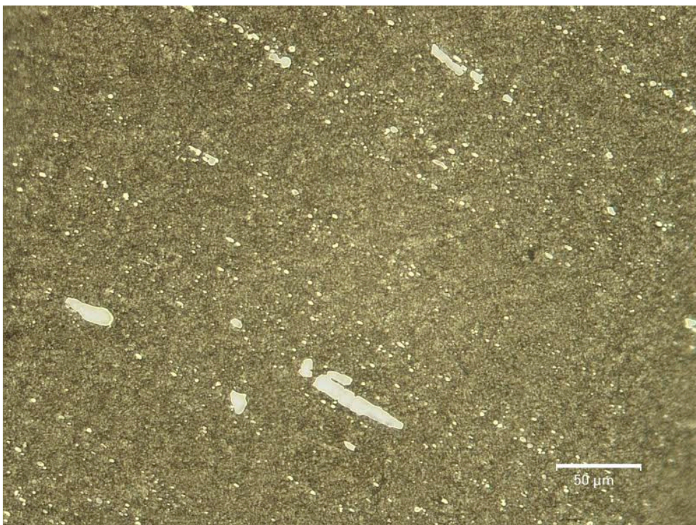
Fig 12. Microstructure of commercial steel austenitized at 1025 °C for 1 hour and tempered twice at 525 °C for 30 minute
