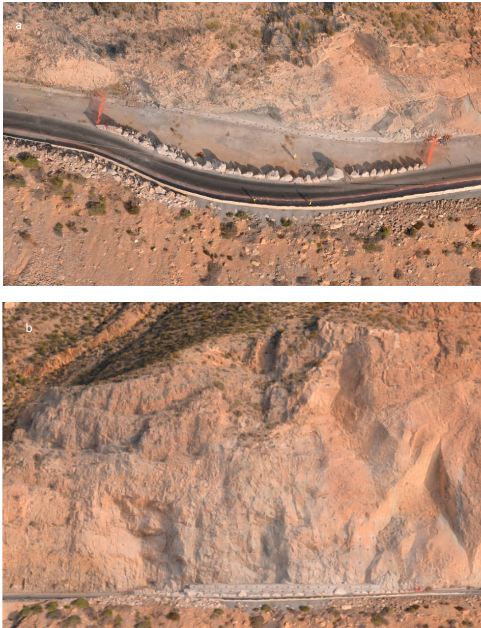
Figure 8. Orthophoto obtained using a horizontal plane (a) and that obtained using the fitted plane (b).
