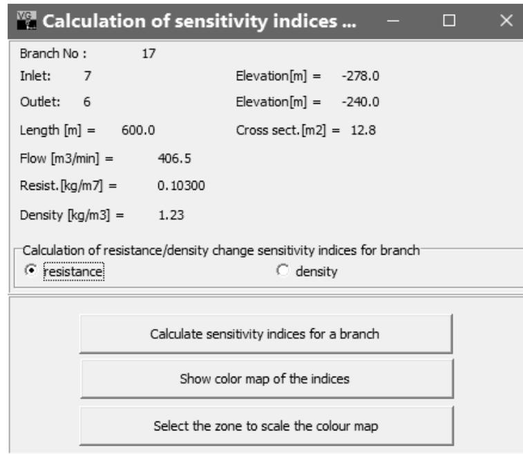
Fig. 3. Calculating sensitivity indicators for branch 17.
