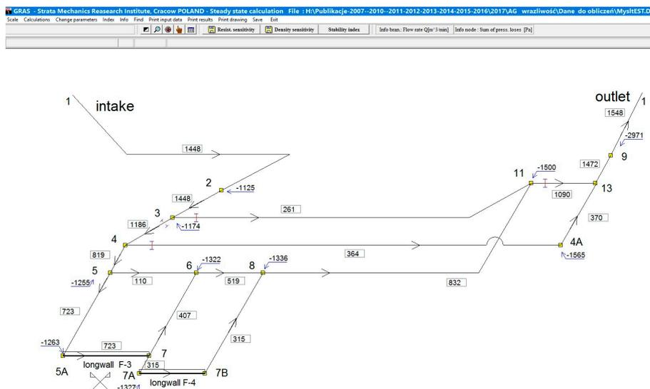
**Fig. 1.** *VentGraph* program window, GRAS module in rectangles – air flow volume stream, in nodes – potential (relative pressure) values.
