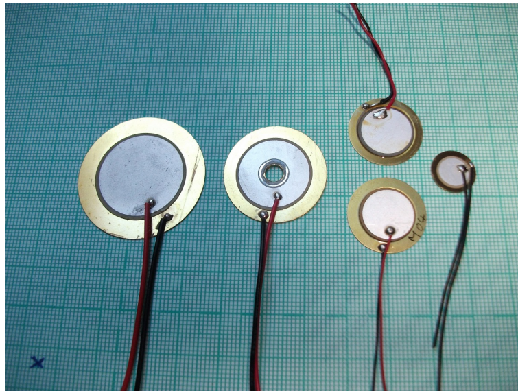
Figure 1. A selection of piezoelectric diaphragms, from left to right - 35mm diameter, 27mm with drilled hole, 20mm diameter salvaged unit from greeting card on top, Murata unit below, 12mm salvaged unit on right.
