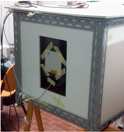
Figure 11. Experimental setup for the laboratory evaluation of U-value of DSM.
