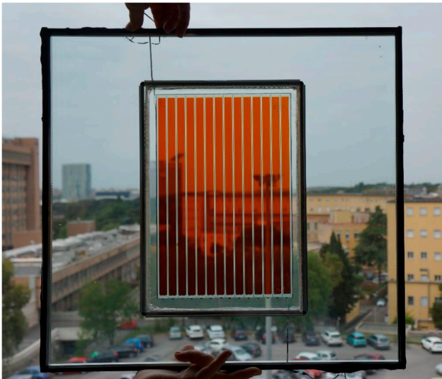
141 142 Figure 2. The glass system prototype used to test DSM with STB; the red stripes are the dye cells connected to 143 form the dye sensitized module.
