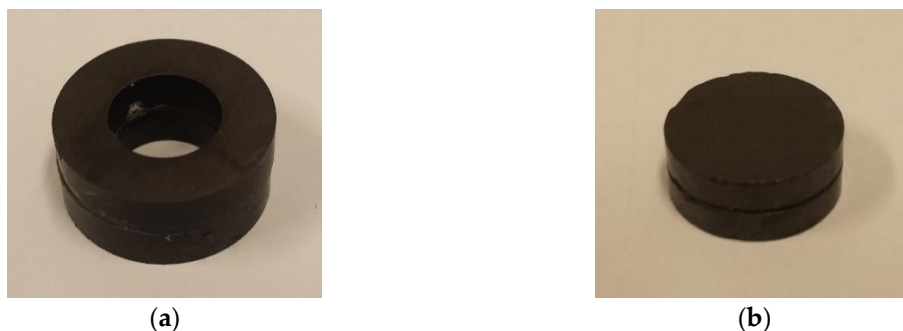
Figure 2. Magnetic quadrupoles used: a) Neodymium rings of 3.5 cm of diameter; b) ceramic magnets of 1.5 cm of diameter
