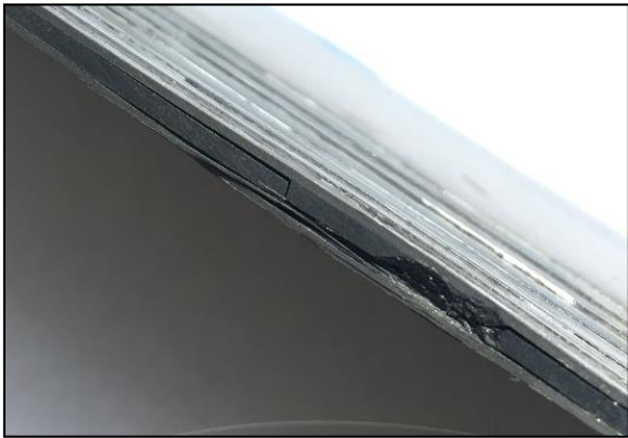
Figure 4. Delamination caused at a (0 4 , 90 4 )s CFRP laminate after a 5 J on-edge impact.
