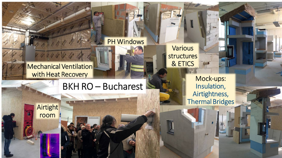
Figure 16. Practical training facility for nZEB in the Building Knowledge Hub (Bucharest).
