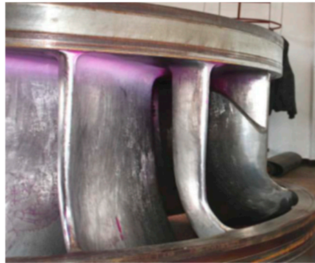
Figure 1. Francis turbine blade failure case reported by D Frunzäverde, 2010[2].
