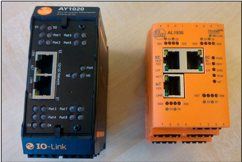
Figure 5. IoT enabled IO-Link gateway to the right, the old one used for this application to the left.
