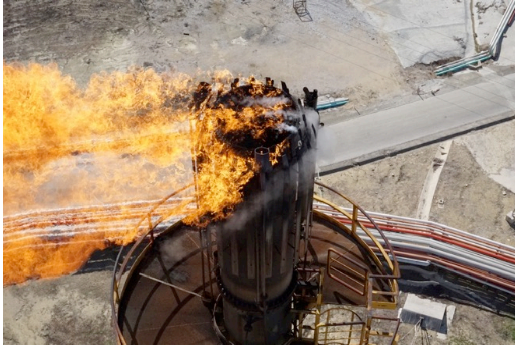
PHOTO 9. Image from above the burner area (tip) of a flare stack with a defect in the steam seal using a drone
