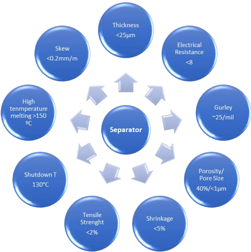
Figure 2 - Main requirements of a separator membrane.
