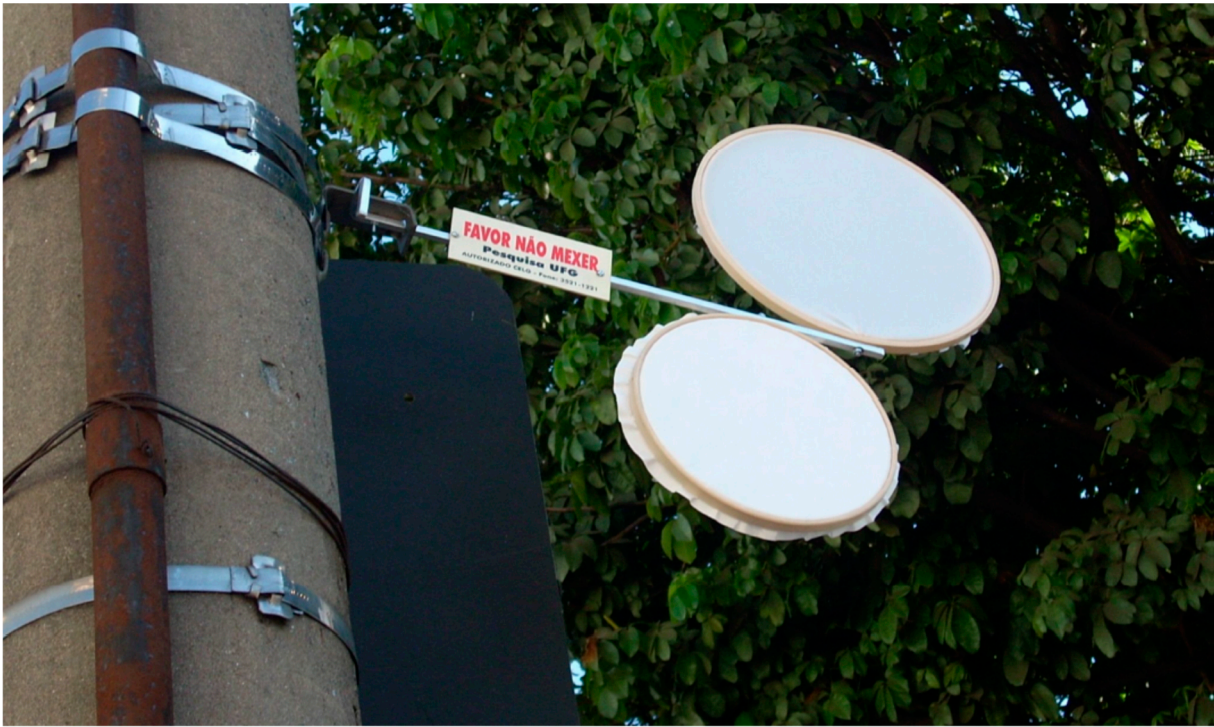
Figure 1. Passive monitoring system mounted with a 0.25-inch aluminium bar and two frames for embroidery in wood, where adsorbent elements were fixed, mounted on a power pole.
