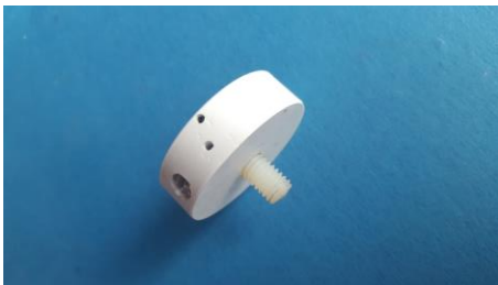
Figure 3. Photo of a PVC-sample with drilling for thermocouples
