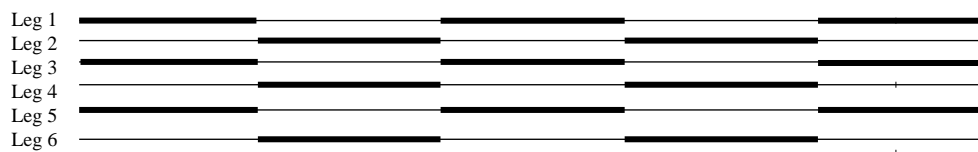
Figure 6. 3-3 gait diagram of 3-UPU hexapod walking robot
