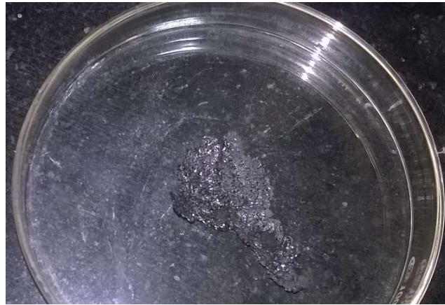
Figure 5 - Flake like structure of powdered Expanded Graphite, Lauric acid and Stearic acid after microwave acid treatment
