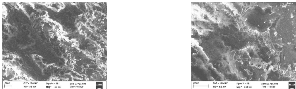
Figure 4 - SEM analysis after microwave treatment of the powdered sample, at different magnifications; Low magnification (Left image), High Magnification (Right image )
