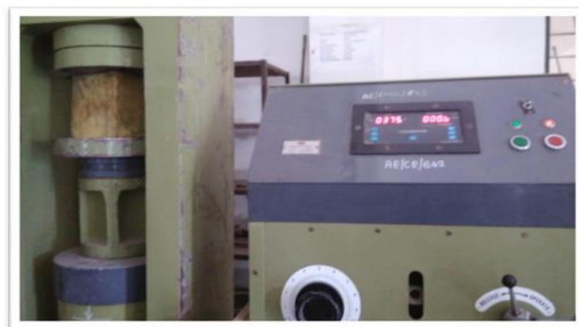
Figure 2. Compressive strength test
