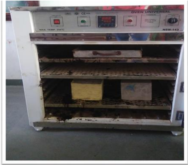
Figure 5. Fire Resistance Test.
